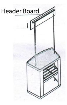
**Step 4:**Slide the header board on to the top of the poles.
