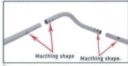
Assemble the two long curved and long straight sections (Connected with bungee cord).
